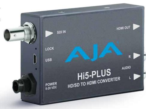
Hi5-Plus is AJA's next generation SDI-to-HDMI Mini-Converter. Capable of handling 3G and Dual Link inputs, Hi5-Plus outputs Deep Color 30 bit video for driving HDMI monitoring solutions. 1080psf inputs are converted to 1080p formats for HDMI compatibility. Embedded audio is user configurable and is passed through to the output and a 2-channel RCA analog output.
